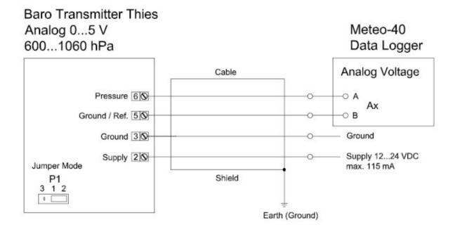
HT0 Jumper P1: 1-2 / PS2 Slope: 92 Offset: 600
